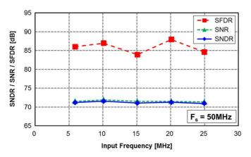
Fig. 22. Measured SFDR, SNR, and SNDR versus input frequency (Decimated by 2).
