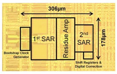
Fig. 19. Die microphotograph of prototype ADC.
