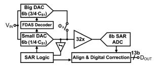
Fig. 6. Proposed ADC architecture.
