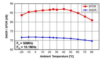
Fig. 25. Measured SNDR and SFDR versus ambient temperature (decimated by 2).
