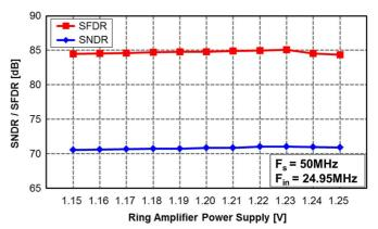
Fig. 24. Measured SNDR and SFDR versus ring amplifier power supply (Decimated by 2).
