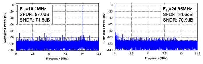
Fig. 21. Measured spectrums for 10.1 MHz and 24.95 MHz inputs sampled at 50 MS/s (Decimated by 2, 65536 point FFT).
