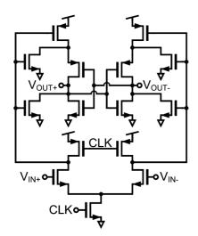
Fig. 17. Low noise single phase dynamic latched comparator [23].
