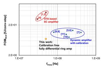
Fig. 2. Walden FOM comparison with conventional SAR-assisted pipeline ADCs.
