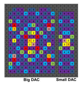
Fig. 18. Common centroid first-stage CDAC layout map. The letter A stands for the feedback capacitors for amplification, D stands for process dummies, 0 stands for the LSB dummies, and the rest of numbers stand for the corresponding bits in 6 bit DAC.
