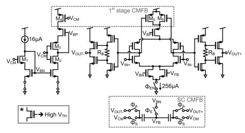
Fig. 5. Fully differential ring amplifier, bias, and CMFB.
