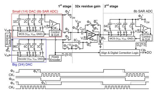
Fig. 16. Block diagram and timing of the prototype ADC (Actual implementation is fully differential).  $CK_1$ ,  $CK_2$ , and rising edges of  $\Phi_{\rm EN}$ ,  $\Phi_{\rm A}$  and  $\Phi_{\rm A}'$  are asynchronously generated.
