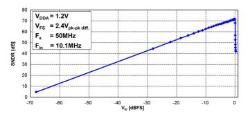
Fig. 23. Measured SNDR versus input amplitude (Decimated by 2).
