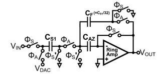
Fig. 7. Residue gain stage structure. Actual implementation is fully differential.
