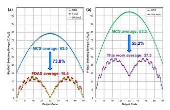
Fig. 13. Calculated 6 bit CDAC switching energy comparison. (a)  $Big\ DAC$  switching energy. (b) The first-stage CDAC switching energy.  $Big\ DAC$  use  $3C_1$  as a unit capacitor and the first-stage CDAC use  $4C_1$  as a unit capacitor. The CDACs uses  $V_{\rm DD}$  and ground as references.
