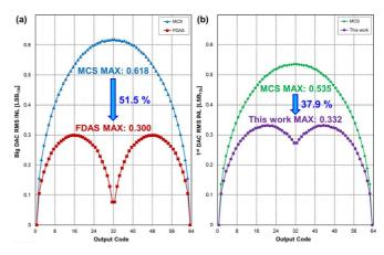
Fig. 15. Simulated RMS INL due to the first-stage CDAC mismatch with 10k iteration and a one sigma  $C_1$  mismatch of 0.3 %. (a) RMS INL due to  $Big\ DAC$ , (b) RMS INL due to the first-stage CDAC.  $Big\ DAC$  use  $3C_1$  as a unit capacitor and the first-stage CDAC use  $4C_1$  as a unit capacitor.
