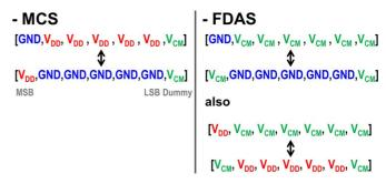
Fig. 14. Worst case INL of 6 bit CDAC switching for MCS and FDAS.
