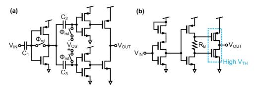
Fig. 3. Conventional ring amplifiers. (a) Original ring amplifier [13]; (b) self-biased ring amplifier [14].
